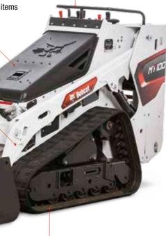
Optional wide tracks reduce ground pressure and increase stability while only increasing width from 904 mm to 1 045 mm
