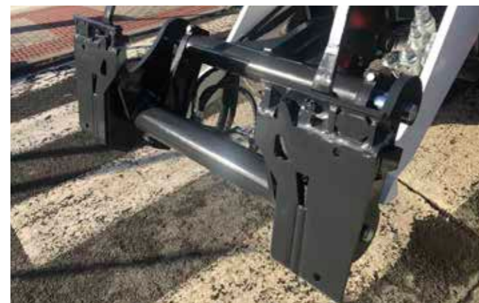
Quicktatch to Bob-Tach adapter (required for all attachments except buckets and pallet forks)
