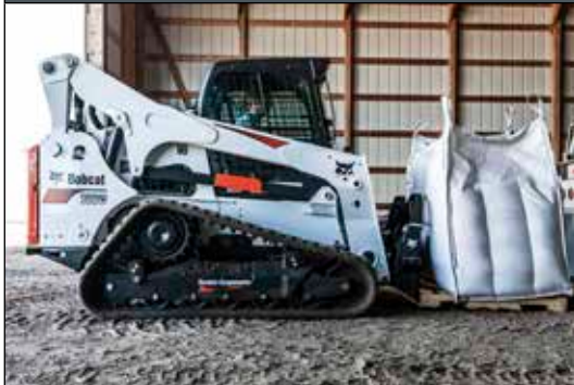
Pallet Forks Standard: Need Mounting Frame & Forks.
