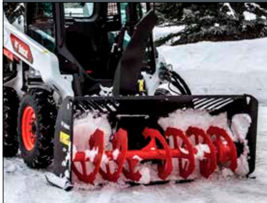
Snow Blower: Includes a hydraulic motor package. Loader must be equipped with a 7-pin Attachment Control Kit.
