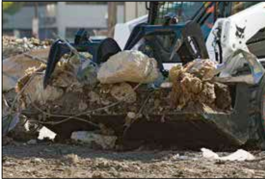
Industrial Grapple: Includes Bolt-On Cutting Edge.
