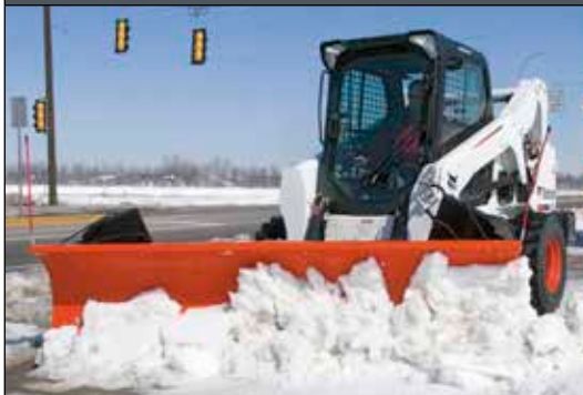
Snow Blade: Includes hydraulic angle.
