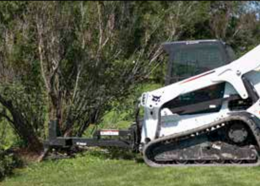
Brush Saw: Special Application Kit must be installed on loader when operating the Brush Saw.
