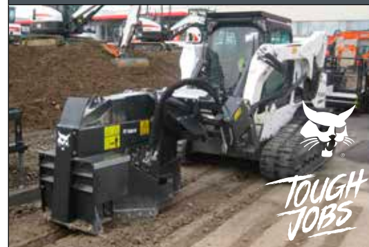
Wheel Saw: For High Flow (H) machines only.
