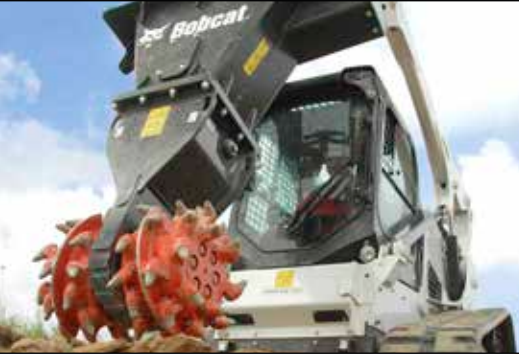
Rotary Grinder: Needs Adapter Frame + Rotary Grinder + 2 hose kits.
