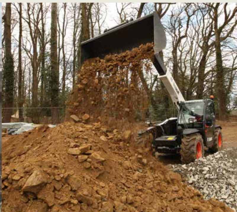
Buckets: for digging or light material handling
