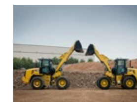
Optional High Lift for increased reach and lift height
